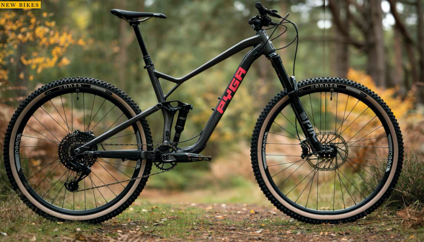
No bridge on the seatstays is good for compliance and clearance
